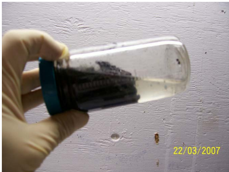
Figure 1 – Dewatering biosolids in a 250-mL sample jar after addition of Solve 9244 (7.4 lb/dry ton) and release of free water.
