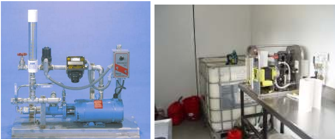
Figure 7 – WaterSolve’s LP5-30 liquid polymer preparation system delivers 30 gpm made-down Solve 152 (left). SIS’s custom polymer make-down unit delivers 10 gph of neat Solve 9244.
